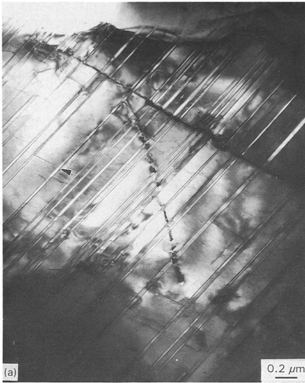
Figure 6 TEM bright-fields of the same area under different beam conditions revealing details of deformation twins and stacking faults. (a) was oriented near a [\bar{1}101] zone-axis; (b) was tilted off the zone-axis to resolve the stacking faults.
