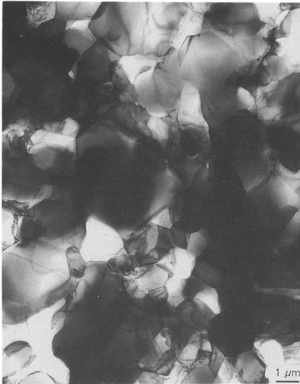
Figure 4 Low magnification TEM of the general microstructure of 65% B 4 C-Al following a shock of 6.4 GPa.
